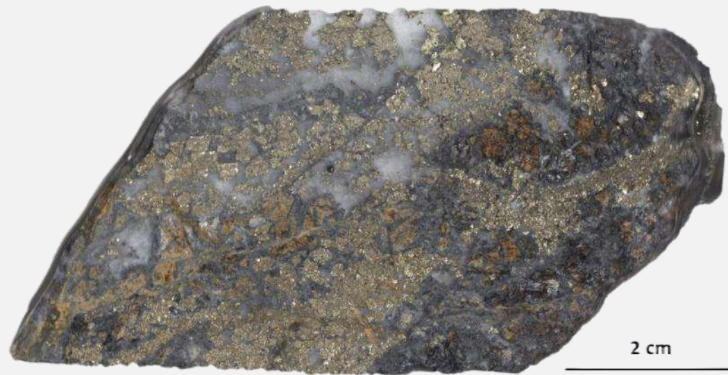
Sulfide vein material from hole NBM88-U28, 177.2-ft down-hole, Lexington-Missoula vein system. 2
